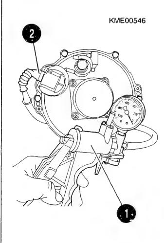
Alternator leak test
